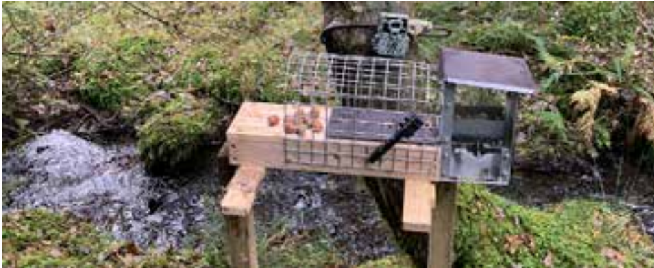
Figure 3a. A grey squirrel selective feeder based on body weight. When a passive infra-red sensor detected movement, the weighing platform was activated. If the weight recorded was at least 450 g, the door to the bait compartment opened. If the weight fell below 450 g, the door closed. The feeder entrance was monitored using a Browning™ Dark Ops Pro X 1080 camera, set to record one photo and one 10 second video per trigger, to identify animals using the feeder.
