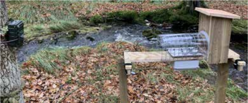
Figure 2a. A red squirrel feeder with integrated automatic weighing scales, designed to record the body weights of red squirrels that feed from it. The weights, together with the date and time they were recorded, were stored on an SD card.
